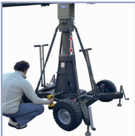
Column extends under full load
