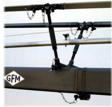
3. Connect 2 x 142cm / 4' 7" rigging rods to the long Rigging Rod Connector. Ensure that the locking pins are inserted fully.
