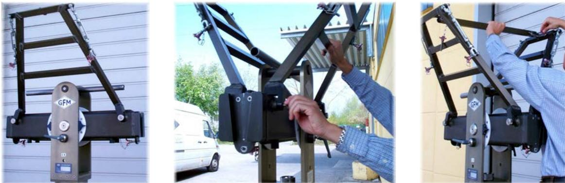
7. For Standard Versions 1 to 16 connect the 127cm / 4ft rear arm section to the middle section. For Standard Versions 17 and 18 connect the 150cm / 5ft section to the middle section. Slip the connection flanges into each other and secure with the provided safety pin.
