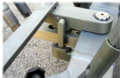
Switch lever (here in upward position)
