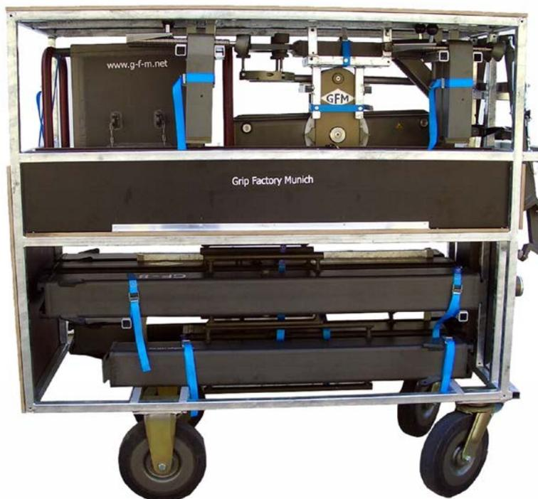
The above photos show the practical transport solution for the GF-8 Crane System. The GFM trolley fits the complete system with dolly and column as an extra unit.
