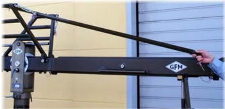
Connecting 1 x 142cm rigging rod to the turnbuckle
