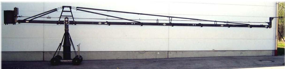
**Attention:** The rigging system of the crane arm should be hand tightened symmetrically from both sides of the crane in a way that the arm is absolutely straight when carrying the loads of the counterweight bracket, the platform or remote bracket.
