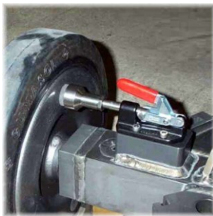
Locked wheel brake on Base Dolly
