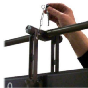
Connecting the safety pin
