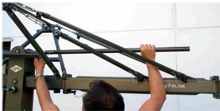
Connecting the parallelogram rod
