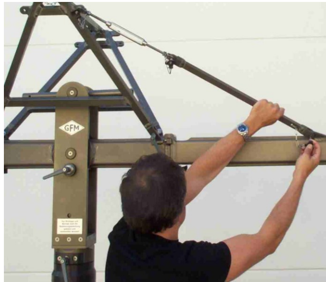
Connecting the rigging rod to extension arm
