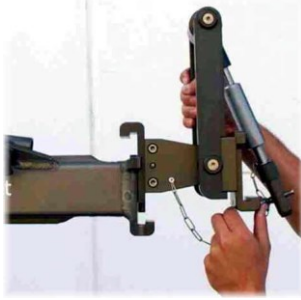
Mounting the angle adjuster
