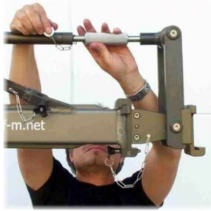
Securing the parallelogram rod
