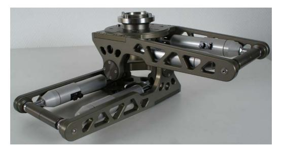
The Iso Dampener increases the efficiency of gyro stabilized heads by reducing rotational stress and smoothening out pan starts and stops on telescopic and fixed arm cranes by isolating high frequency vibrations between the mount and head.
